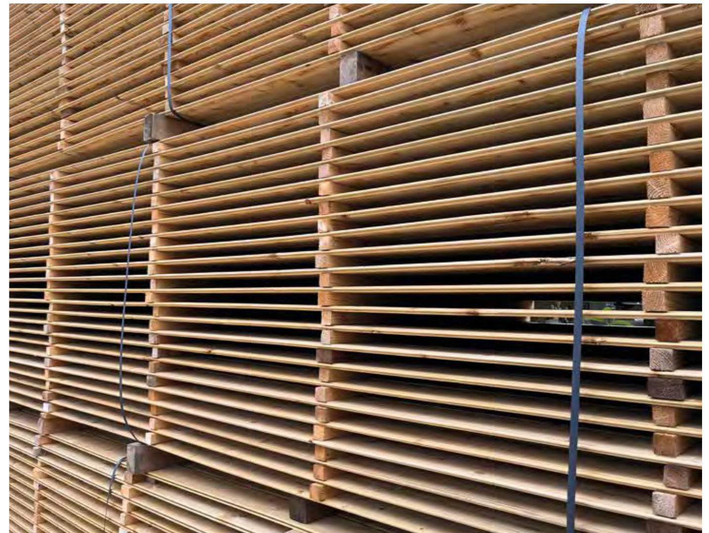
Latted timber drying process
